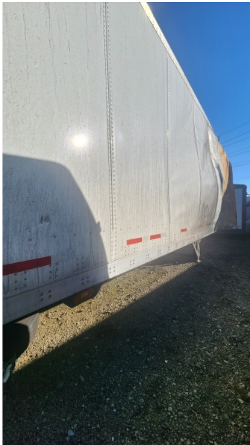
4 sections was damaged on the passenger's side
