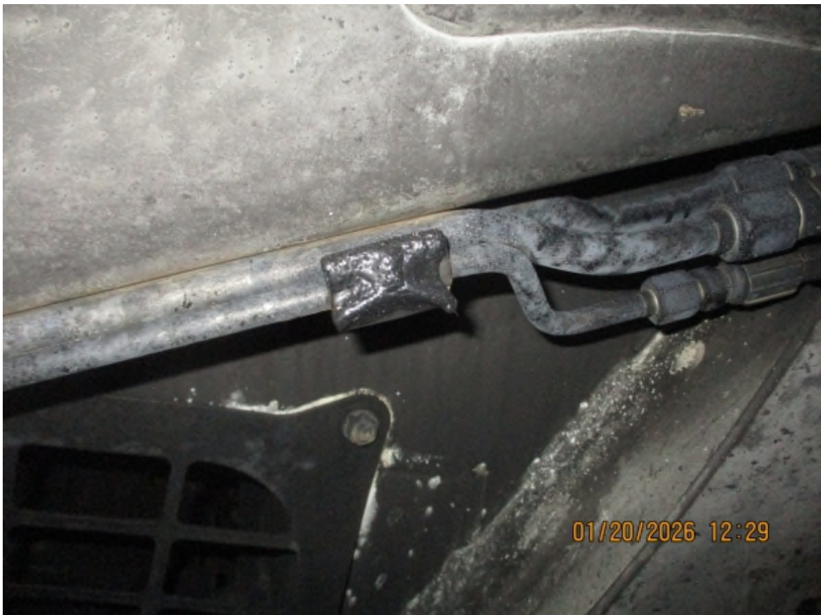
Melted plastic on hydraulic line
