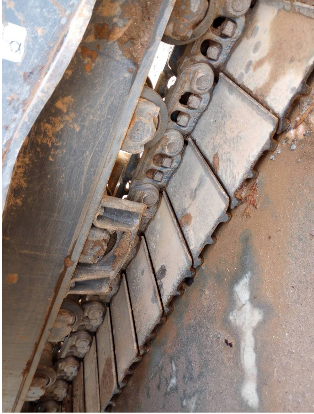
Tracks of 2022 Volvo EC200EL Excavator VIN: VCEC200EH00314700.
