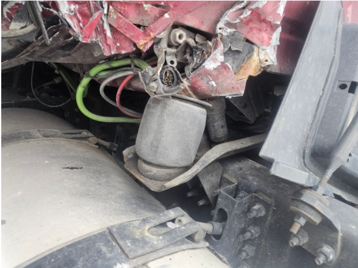
air lines and trailer plug
