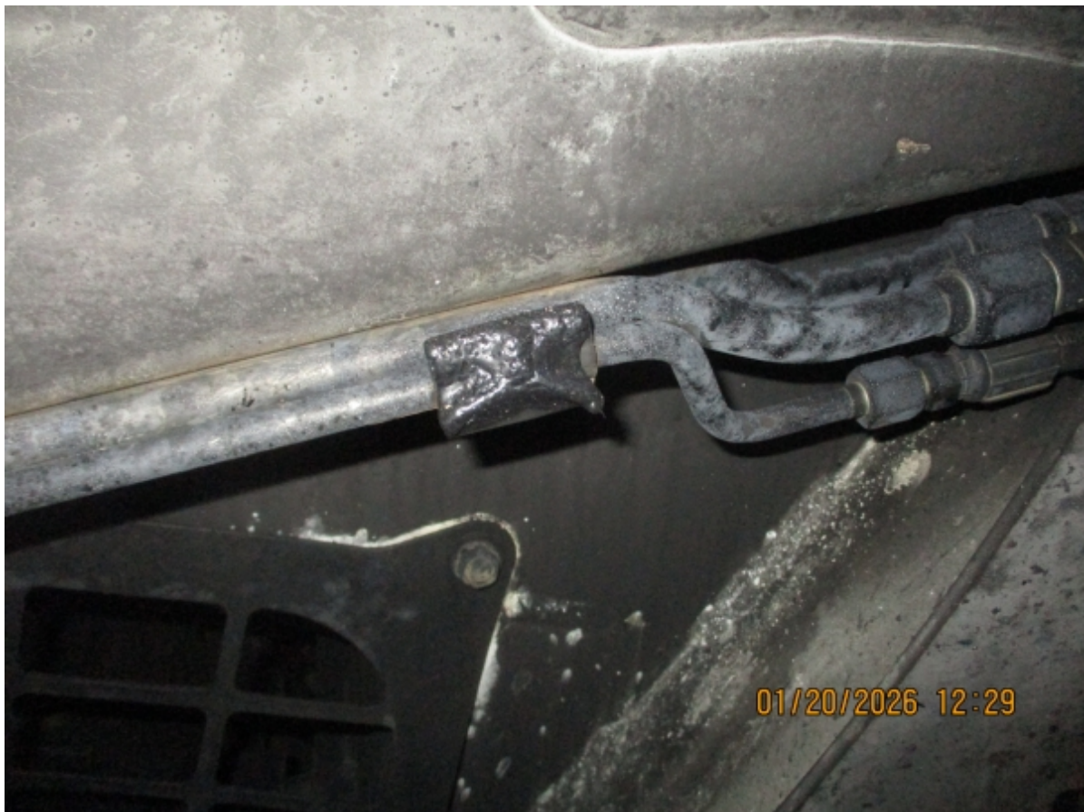
Melted plastic on hydraulic line
