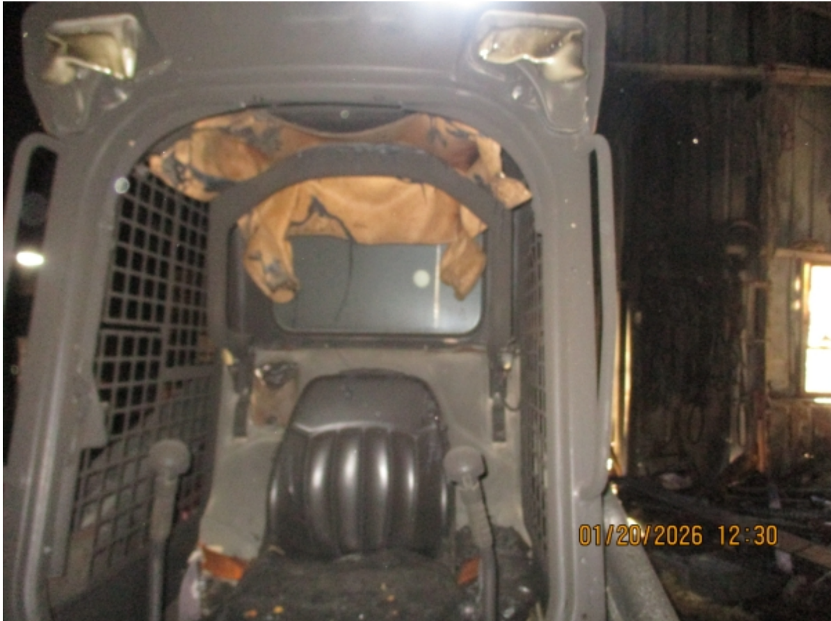
Upper Cab & melted Roof
