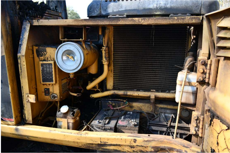
Photo 007: Showing radiator, batteries and air intake with no visible fire effects.
