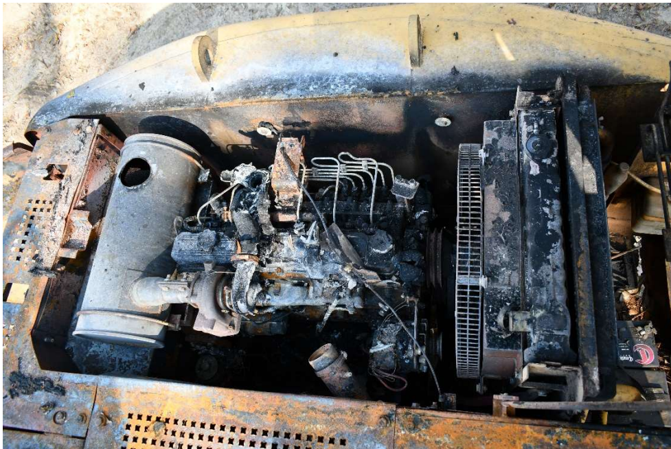
Photo 010: Showing minor mass loss of components on top of engine, fire movement from left to right of photo.
