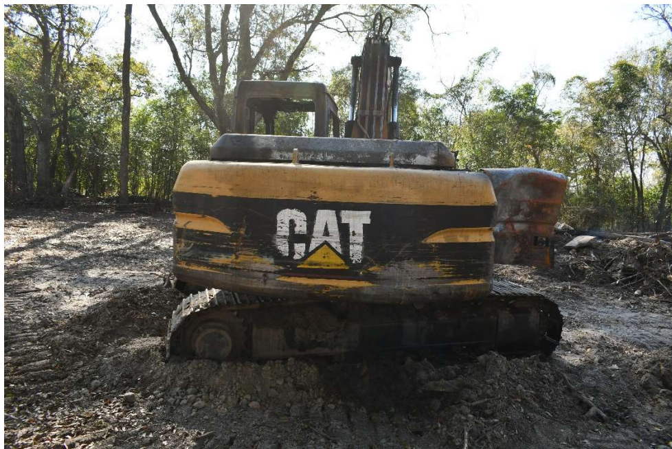
Photo 002: Showing Discoloration and oxidation of engine cover.
