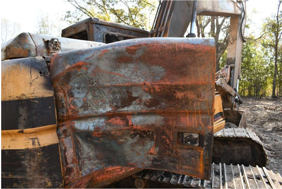
Photo 005: Showing Discoloration and oxidation on hydraulic pump compartment door, area of origin.
