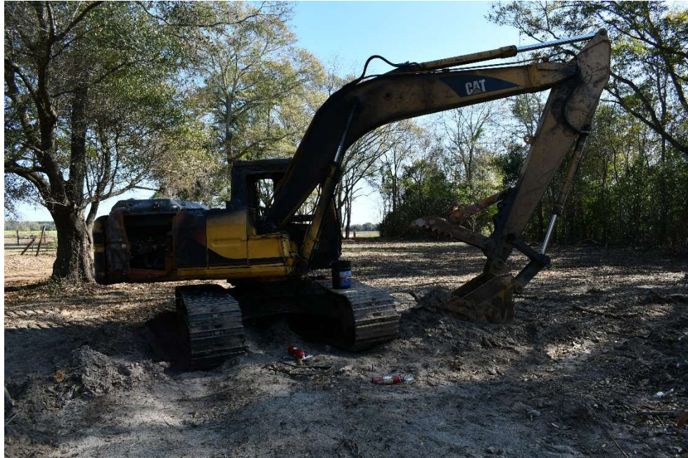
Photo 001: Showing discoloration of boom and rear of excavator.
