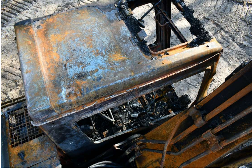
Photo 009: Showing oxidation on cab with mass loss of cab glass.
