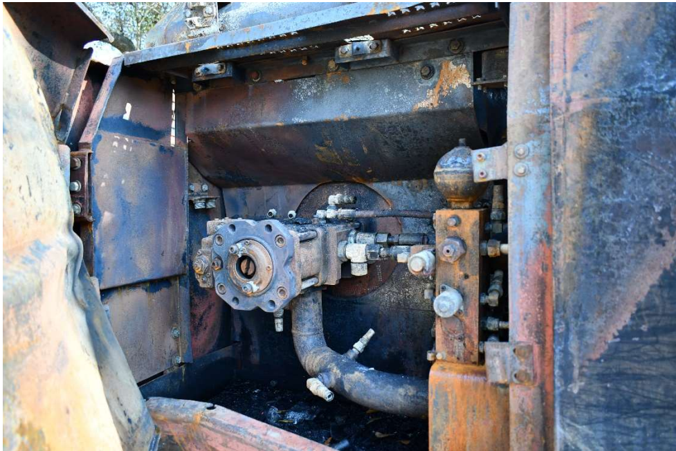
Photo 006: Showing total mass loss of hydraulic hoses and oxidation and discoloration to inside compartment.
