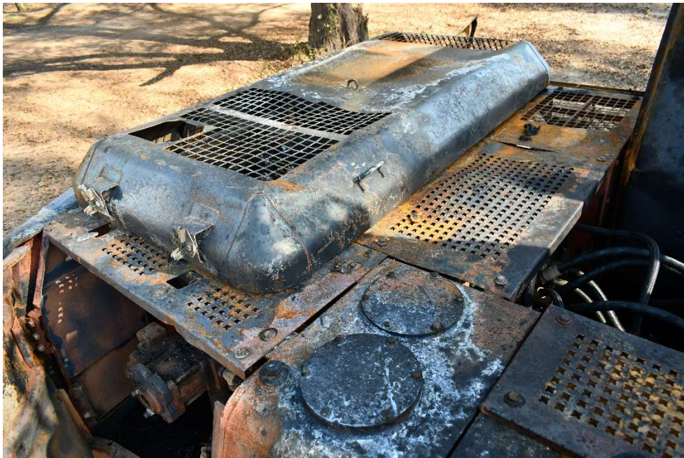
Photo 008: Showing severe oxidation around hydraulic pump compartment extending across the top of engine compartment.
