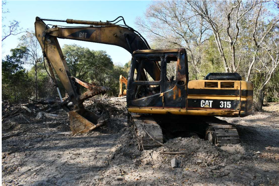
Photo 003: Showing oxidation on cab and mass loss of window glass.
