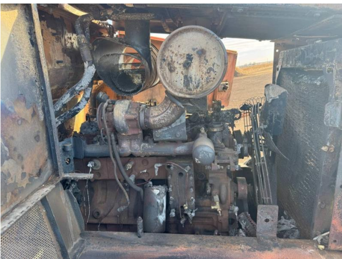
Air intake system, fuel lines, coolant lines, and wiring all damaged.
