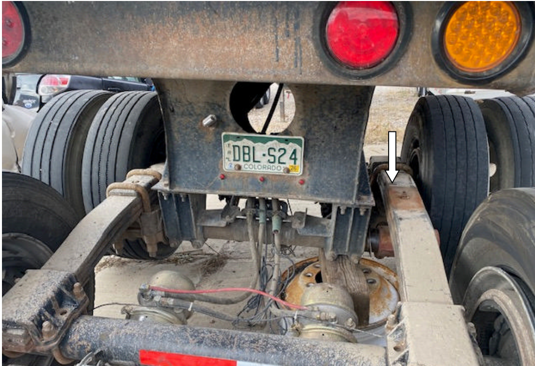
Trailer tag. Arrow indicates missing leaf spring support that failed. Note the two supports on left side.
