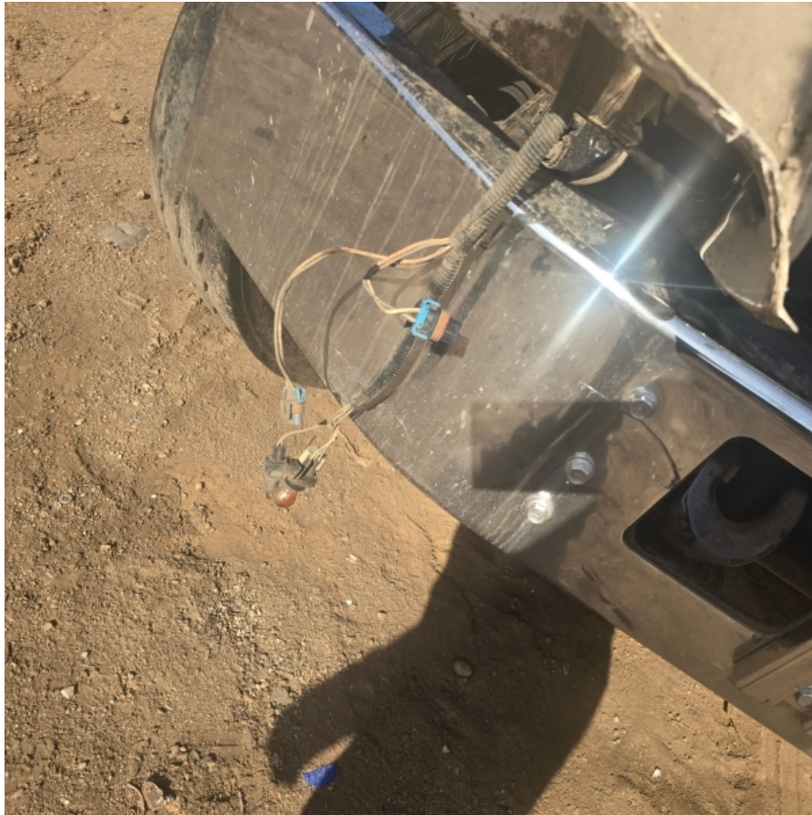
Right Wiring Damage
