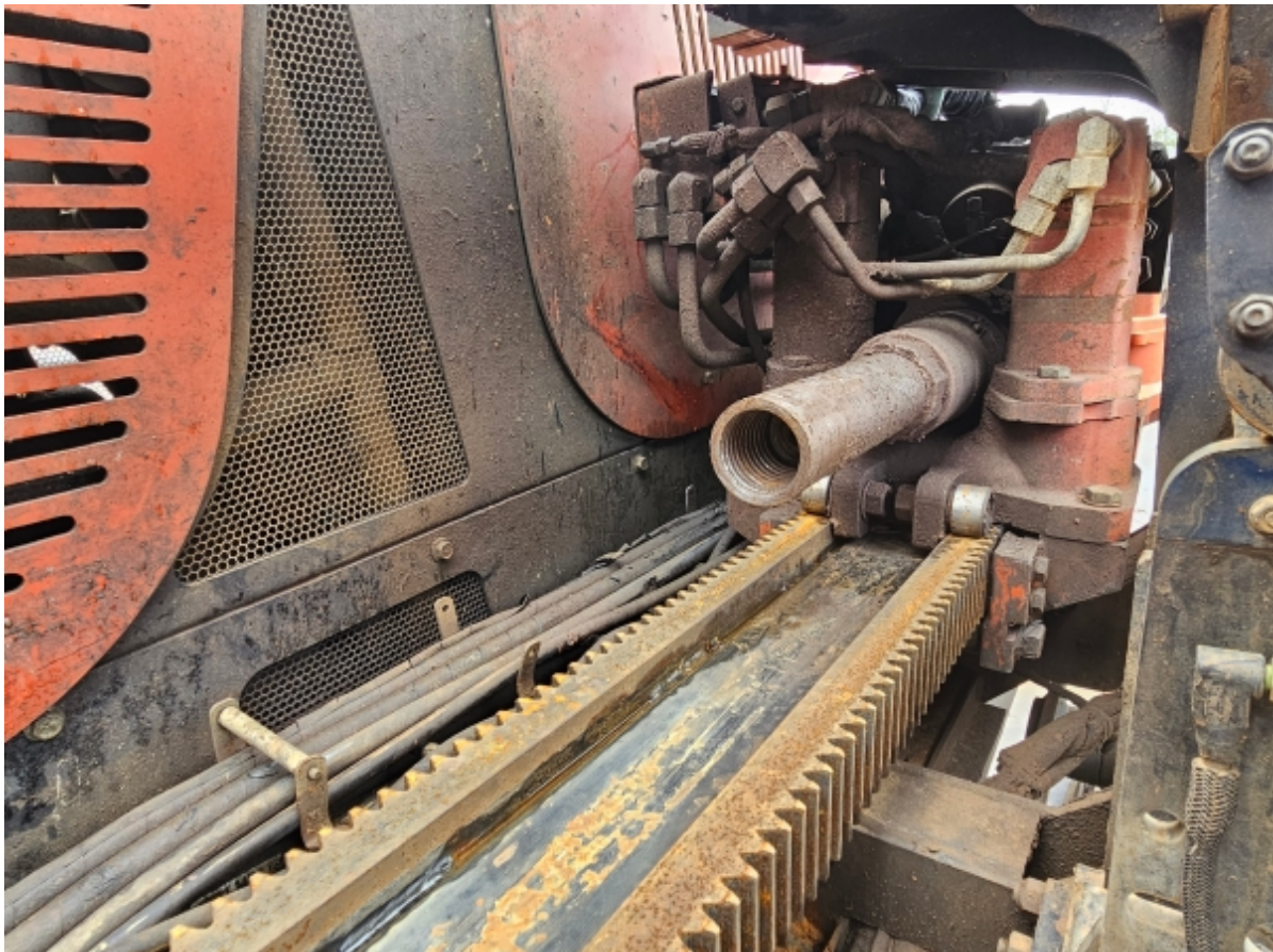
MECHANISM THAT AUGERS PIPE INTO GROUND
