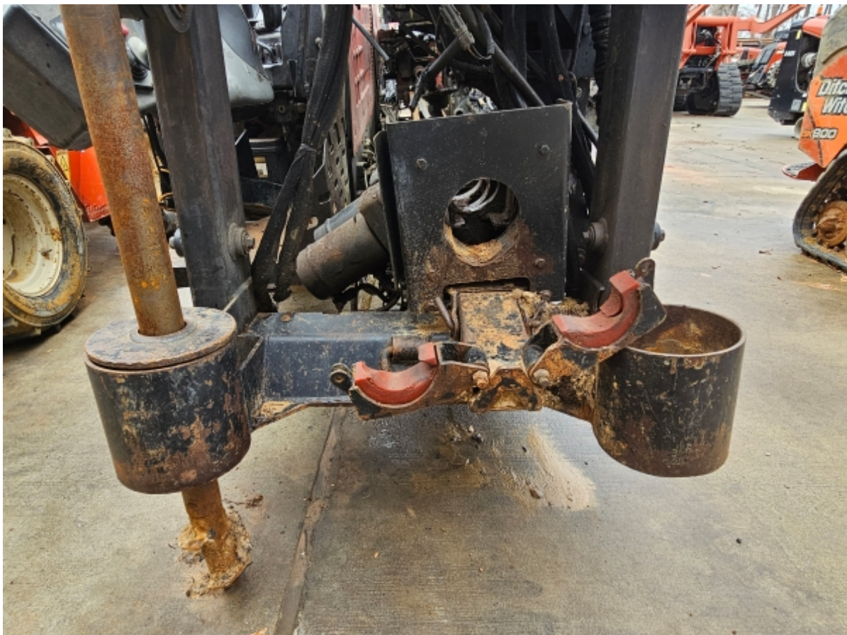
AREA WHERE PIPE EXTENDS IS BENT AND DAMAGED
