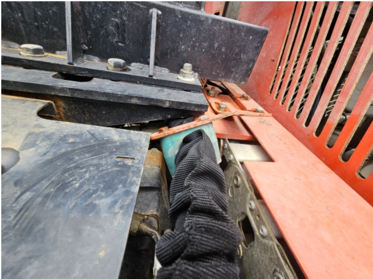
BRACKET IS BENT
