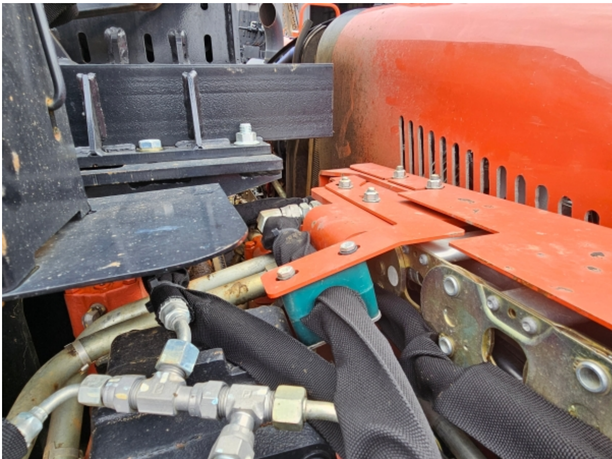
COMPARISON UNIT AS BRACKET AND HOSES SHOULD LOOK
