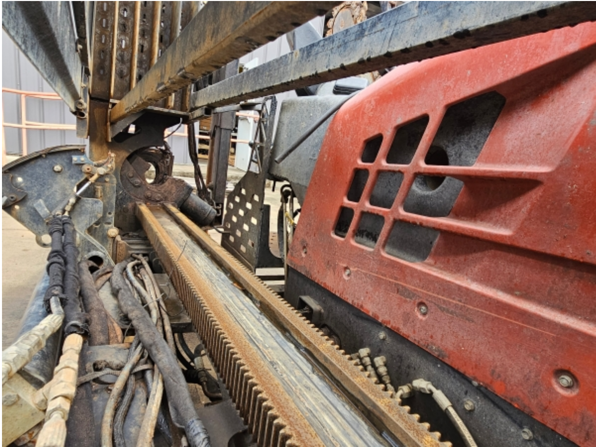
TRACT THAT PIPE GOES INTO AND HOLE MISALIGNED
