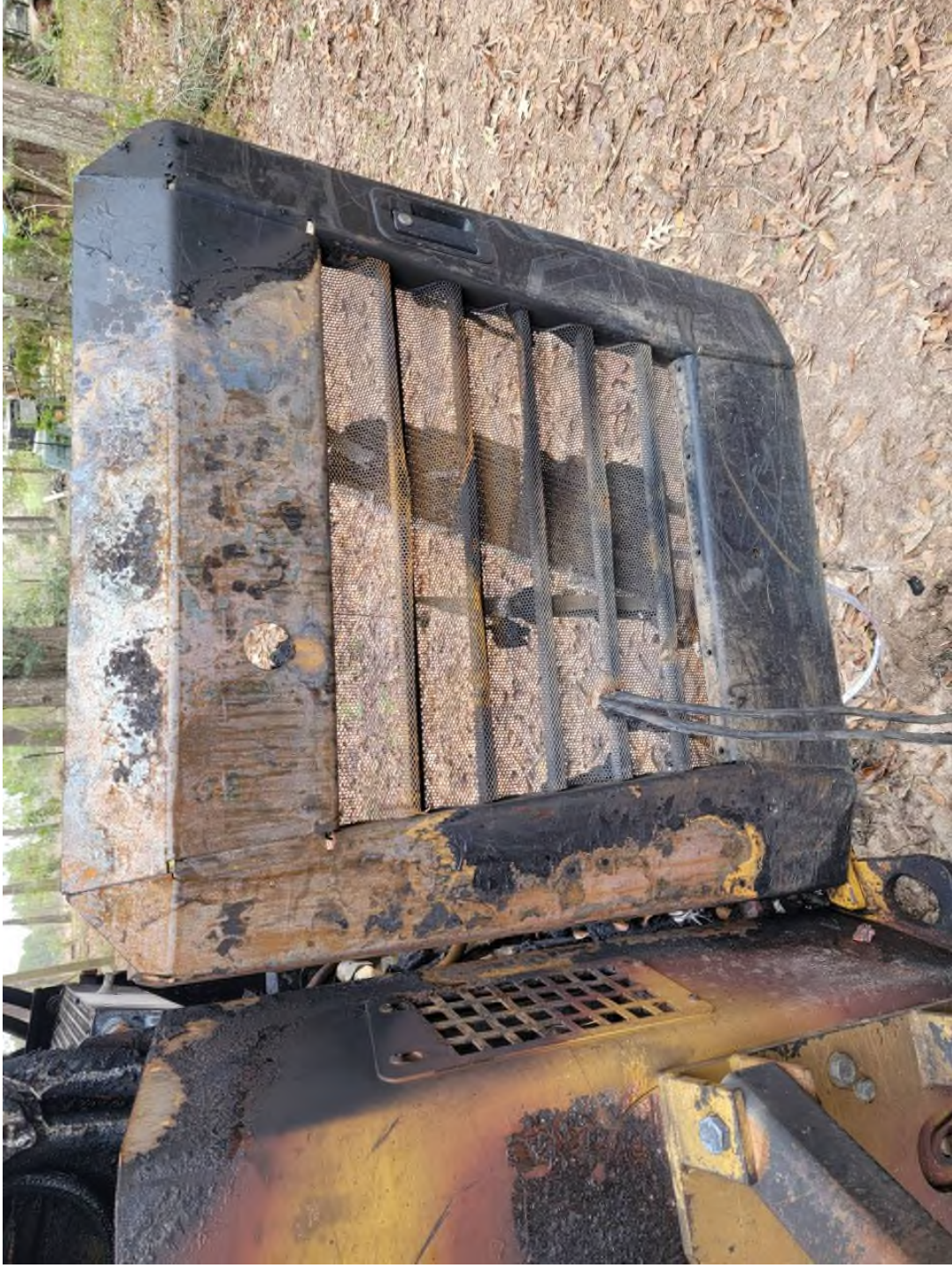
Damage noted to rear of vehicle of 2018 CAT Skid Steer .
