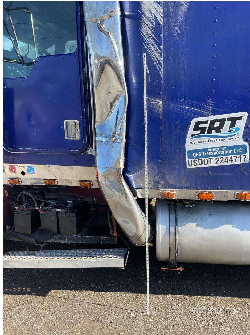
Damage noted to driver side of vehicle of 2000 Blue Kenworth W900 Tractor Plate: IN - 3034376 VIN: 1XKWD9X1YJ816865.
