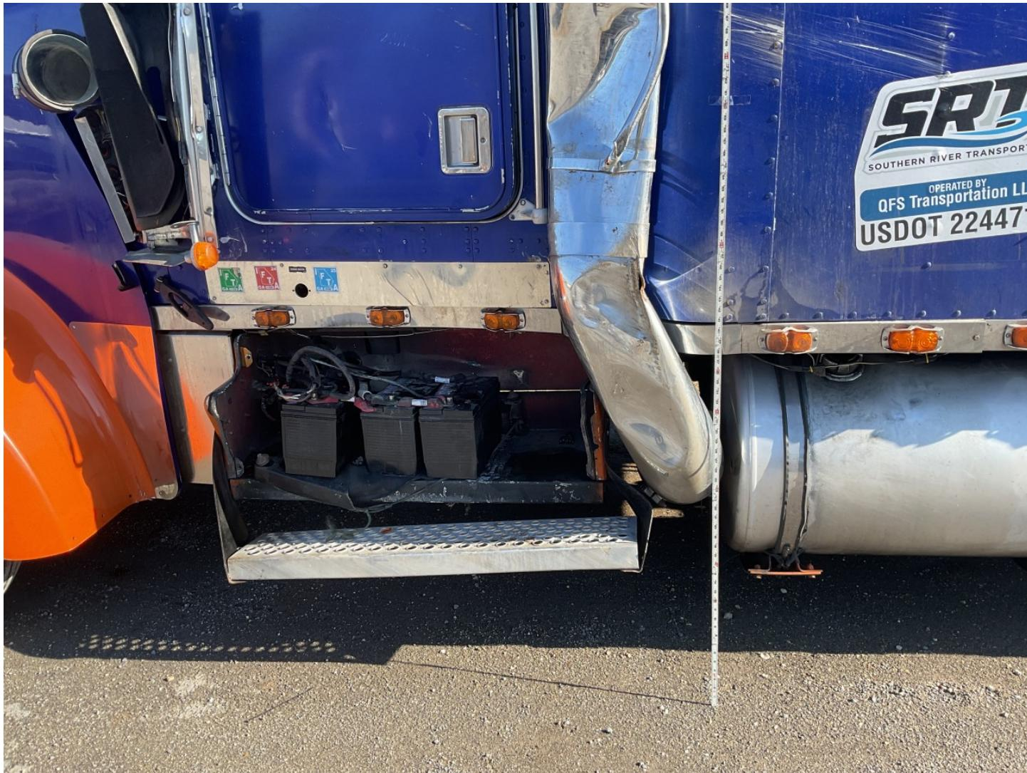
Damage noted to driver side of vehicle of 2000 Blue Kenworth W900 Tractor Plate: IN - 3034376 VIN: 1XKWD9X1YJ816865.
