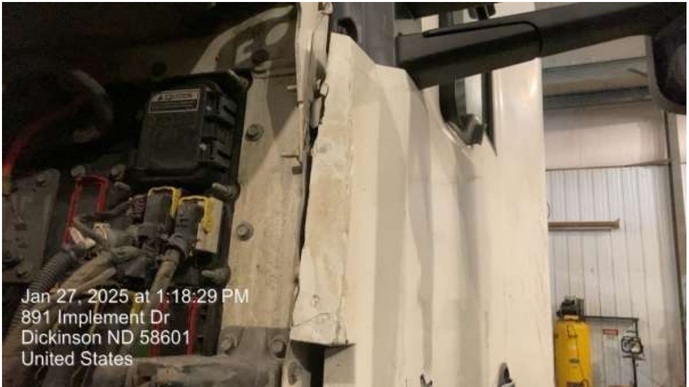
left fender extension cracked
