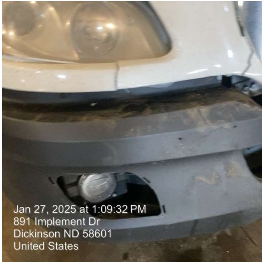
right side cracks in hood
