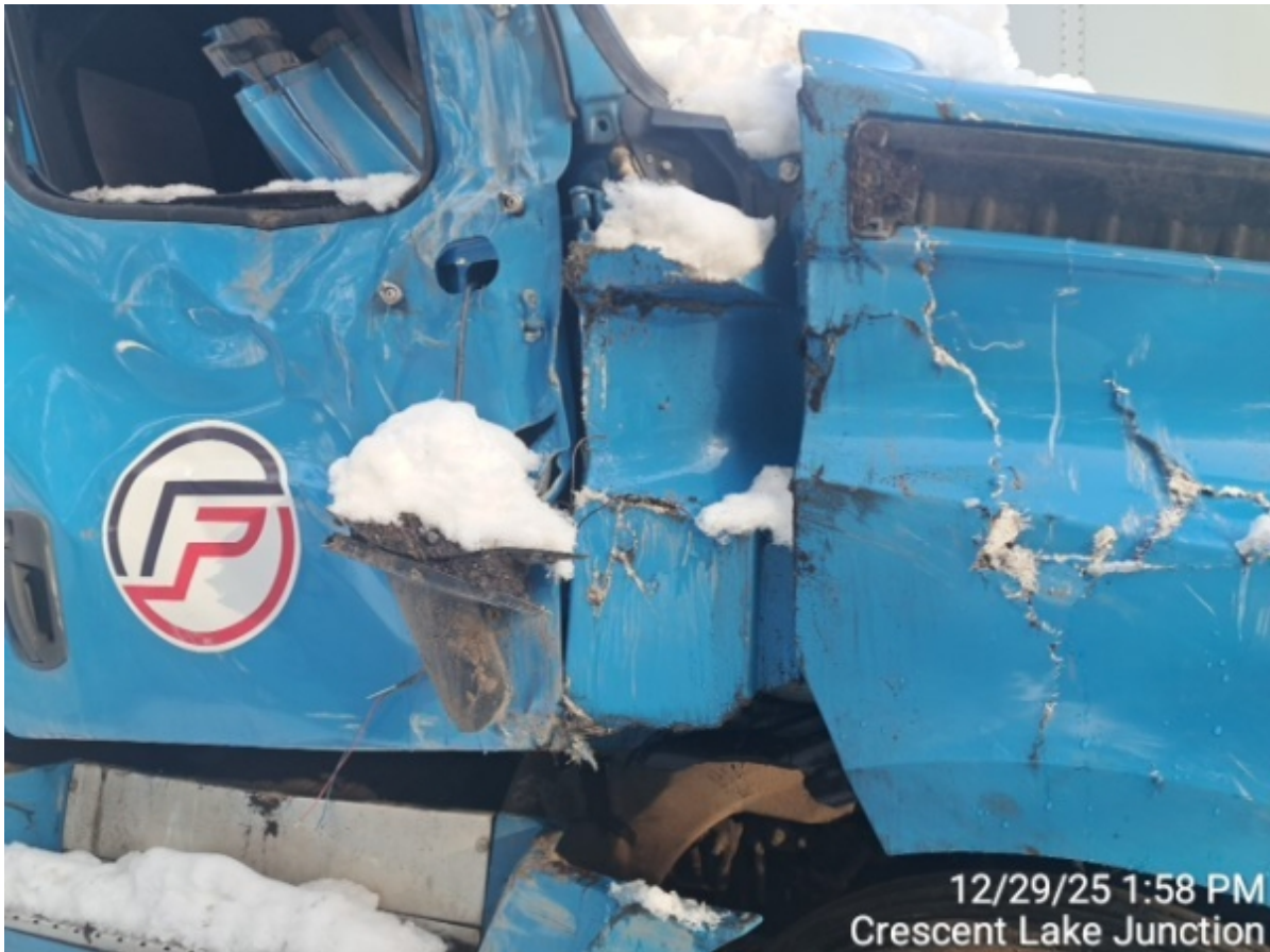
RT FR DOOR DAMAGE
