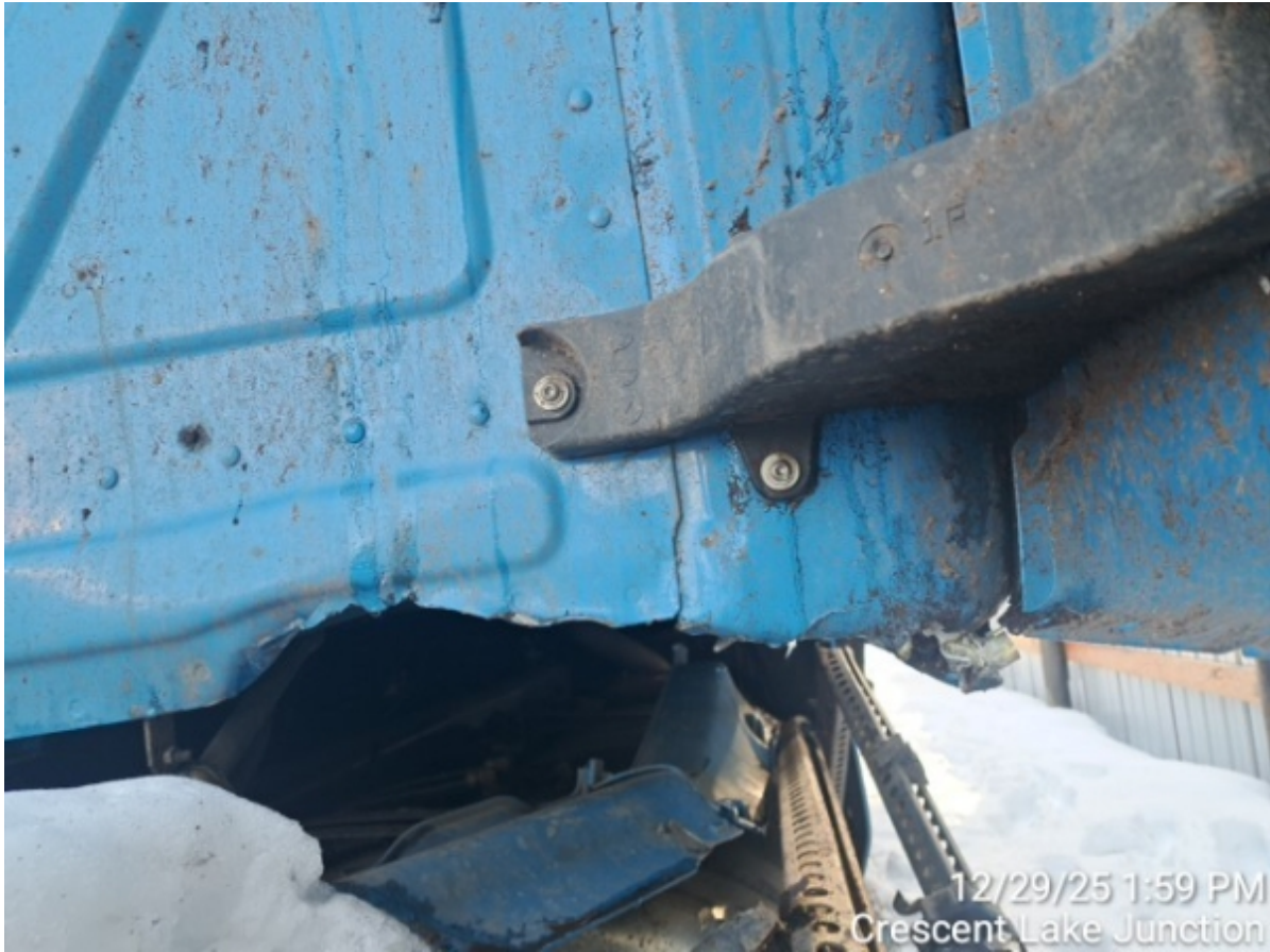
RR PANEL DAMAGE
