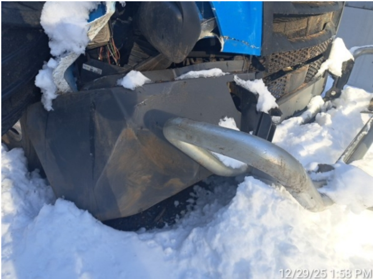
FR BUMPER DAMAGE
