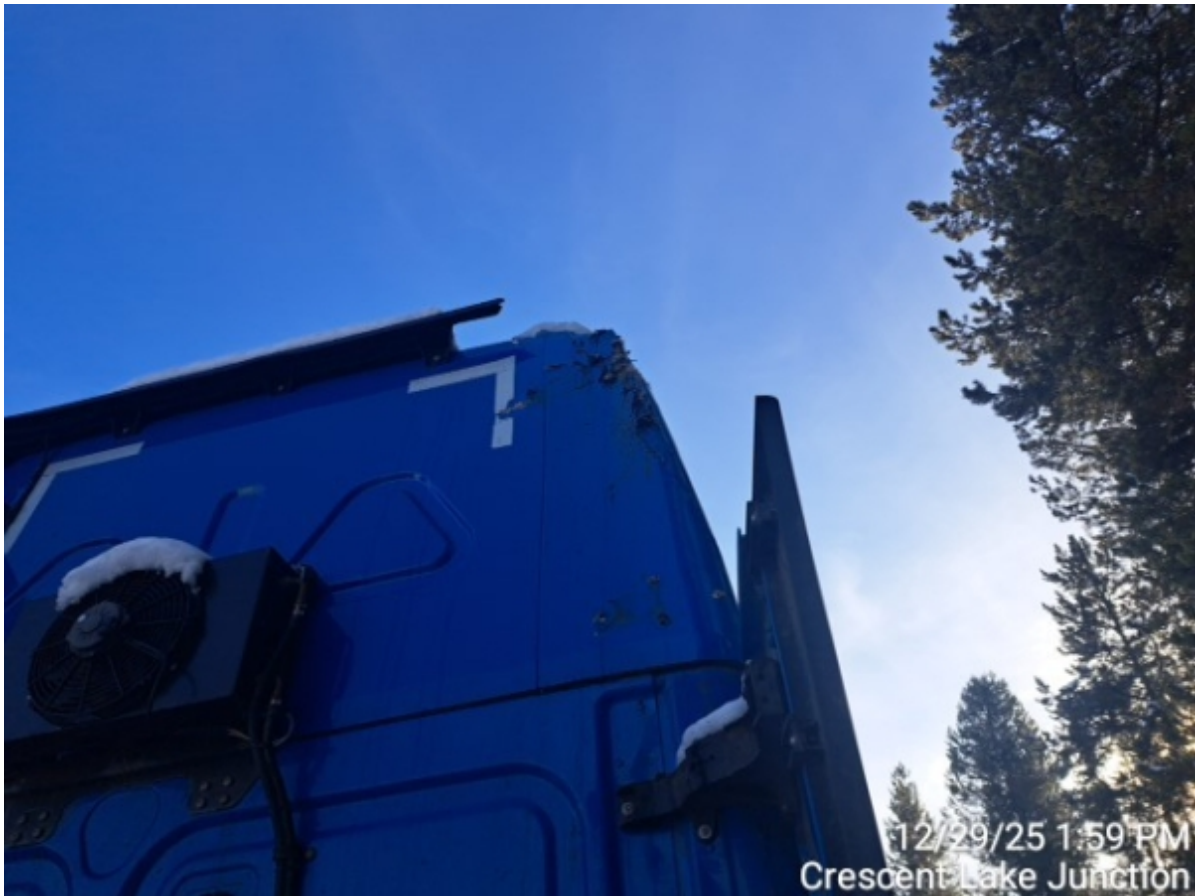
UPPER RR PANEL DAMAGE
