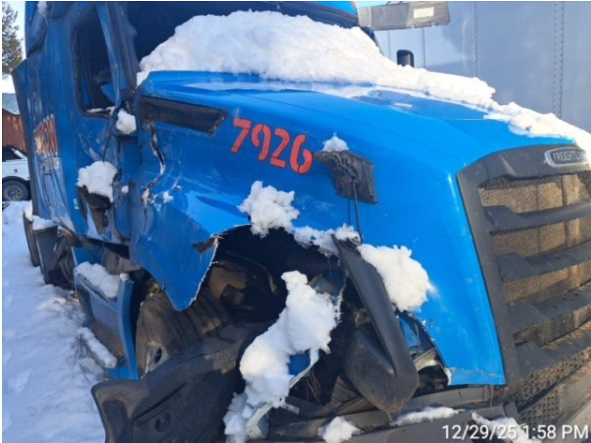
RT FENDER DAMAGE
