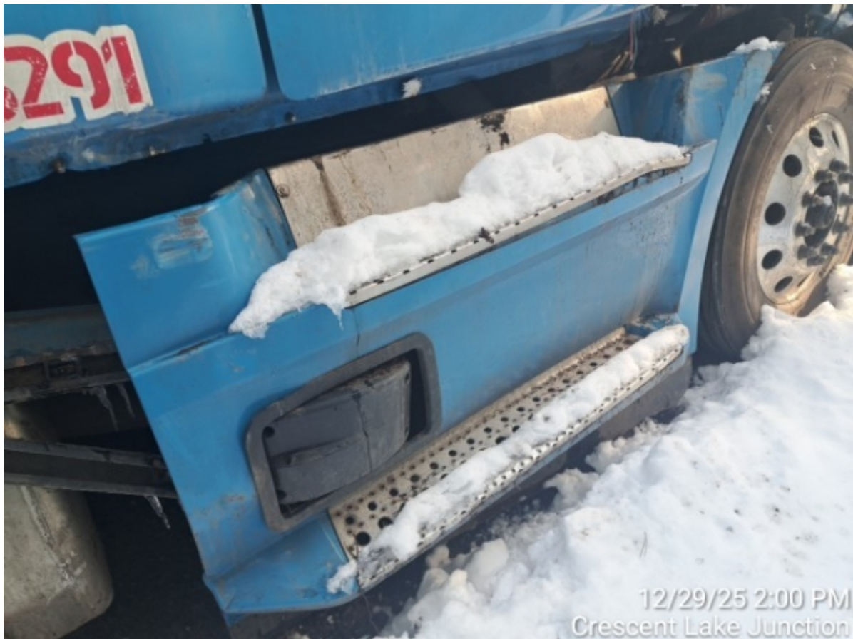
RT SIDE DAMAGE
