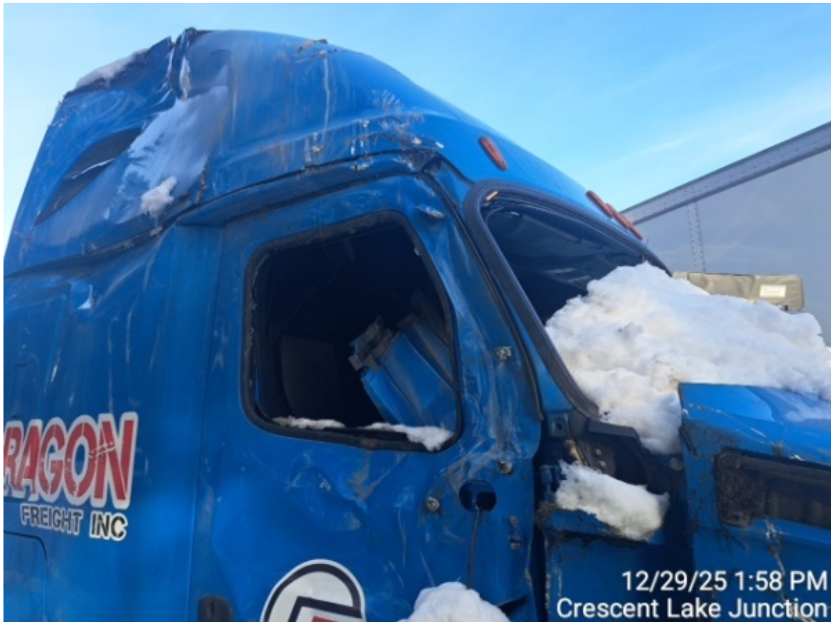
RT CAB CORNER DAMAGE
