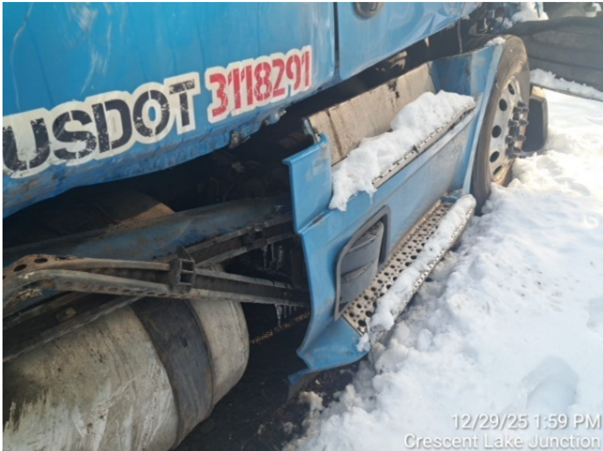
RT SIDE DAMAGE
