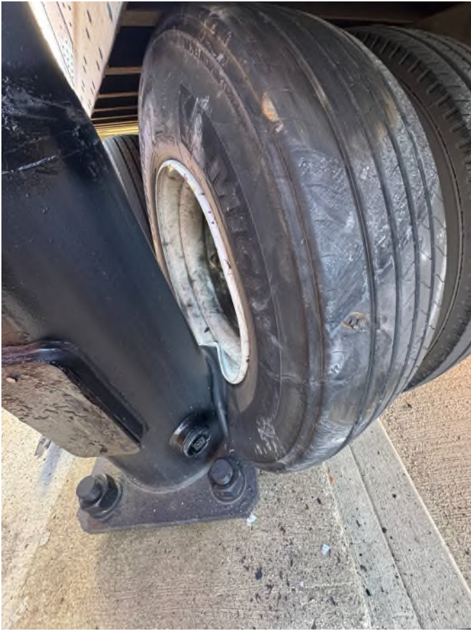
Right Rear Outer Wheel & Tire Damage
