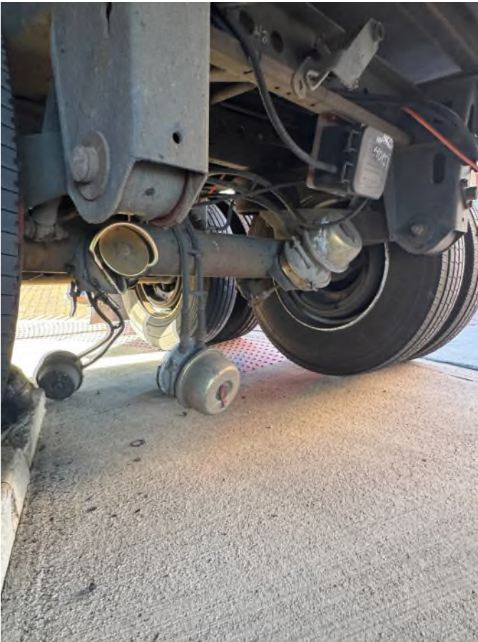
Rear Suspension Damage
